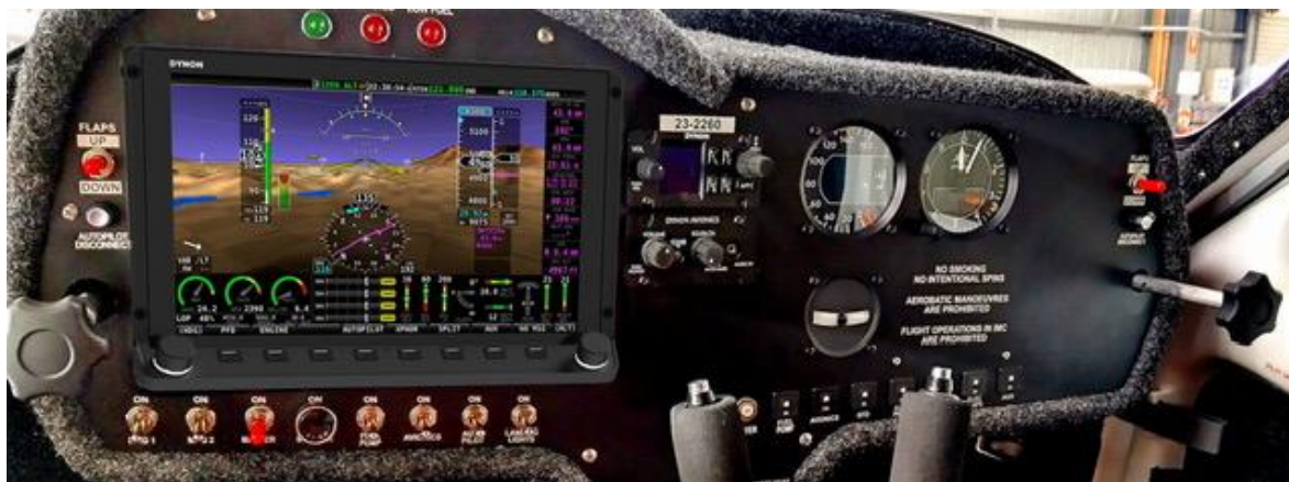
A busy looking panel. Bottom left corner of the Dynon-the little white arrow gives x-wind info
