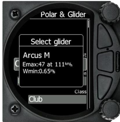
You can modify the polar by changing coefficients **a**, **b** and **c**. A polar is defined as a quadratic equation with the parameters a, b, and c.
