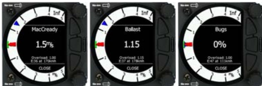
Rotate the bottom knob to modify any setting. Next check the safety altitude (height above destination, arrival altitude) setting.
