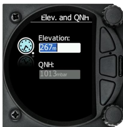
The user must set either the Elevation or the QNH with the lower rotary button. After pressing the lower rotary button, the user can switch between the Elevation and QNH dialogues. As soon as the settings are set the middle button must be pressed to proceed.
