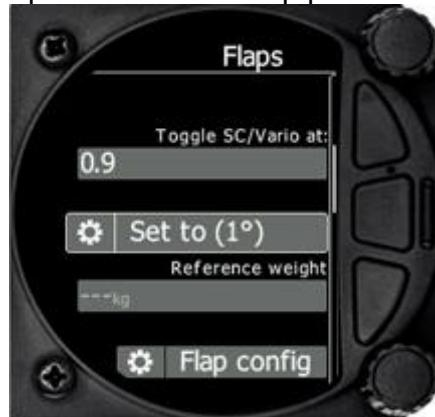
When all flap positions are set, a green dot will be displayed with current flap position. If flap labels are not set yet, press **EDIT** to name label. Flap labels must be entered with increasing speed range. It is recommended that flaps labels are set together with speed range in Polar and Glider setup. It is also possible to toggle between cruise and climb mode using the flap sensor.
