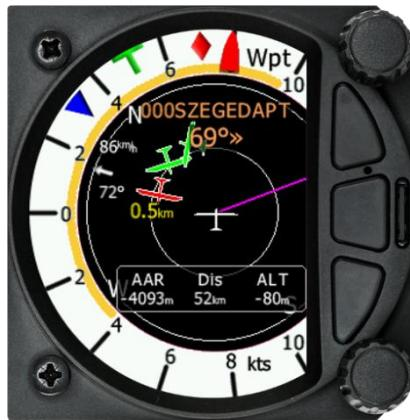
The first page shows a line to a selected waypoint, the name of the selected waypoint at the top of the screen and the relative bearing and chevrons indicating the direction to turn towards the selected waypoint.
