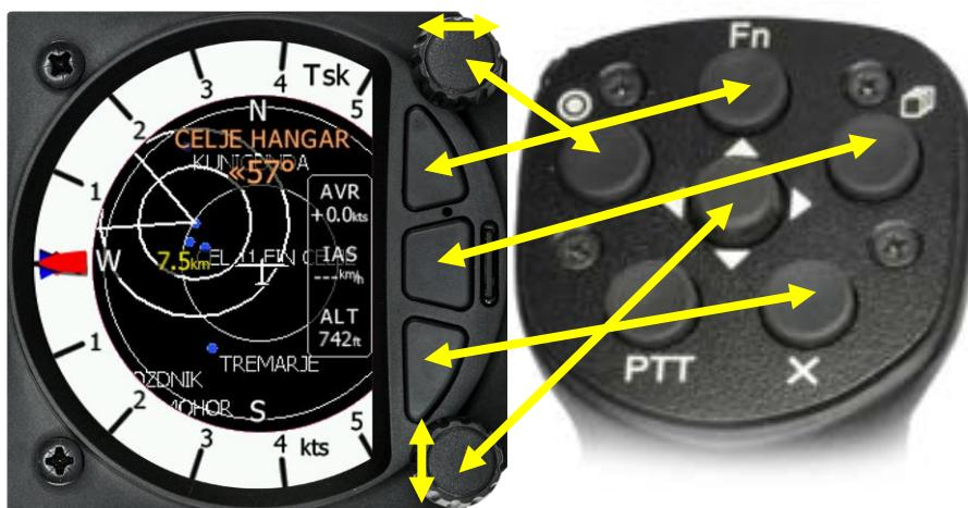
The remote stick is also connected to the CAN bus. On the S8x/S10x a special menu is provided to register the remote stick. The device must be registered in case of two-seat device; it is possible to have two remote sticks, one registered on the front and another on the rear device.
