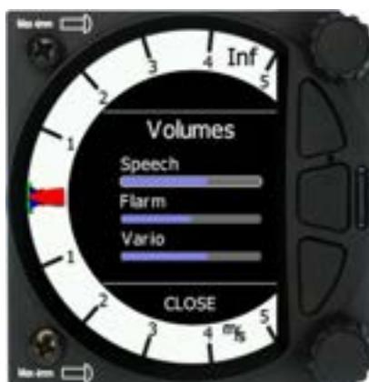
The lower rotary knob is used to adjust settings within the current mode or within menus. With the lower rotary push button, it is possible to toggle between the MC and the Ballast and Bugs settings. In all other menus this knob is used for setting values and editing texts.
