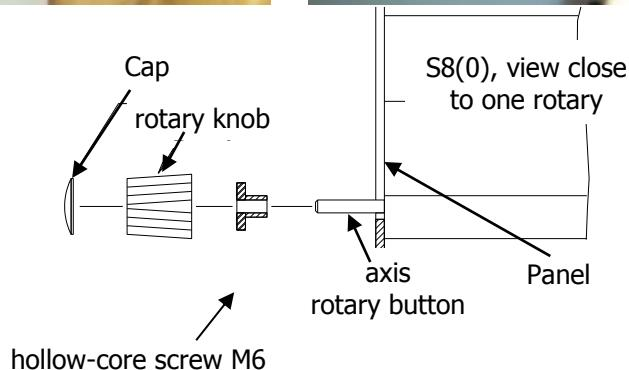
Remove the two rotary knob caps with a knife or flat screw driver, then hold each knob and unscrew it. Remove the remaining two screws and the two M6 threaded nuts. Install the S8x/S10x into the panel and screw back all screws, nuts and knobs. Ensure that between the knobs and the panel there is sufficient space so that the button can be pushed.
