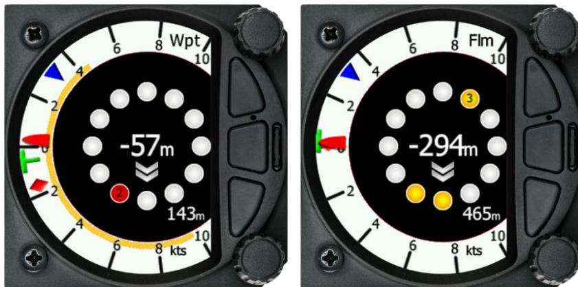
*The central number and chevrons indicate if the Flarm target is below or above and by how many meters/feet. The number in the bottom right indicates the range in meters/feet. The numbers are related only to the closest or the most dangerous target.*
