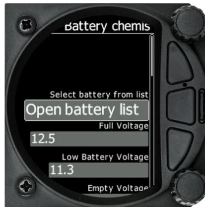
Select battery from list gives you a drop-down list with the suggested battery settings for Full Voltage, Low Battery Voltage and Empty Voltage as pre-sets. Selecting one of these will set the values in the following boxes.
