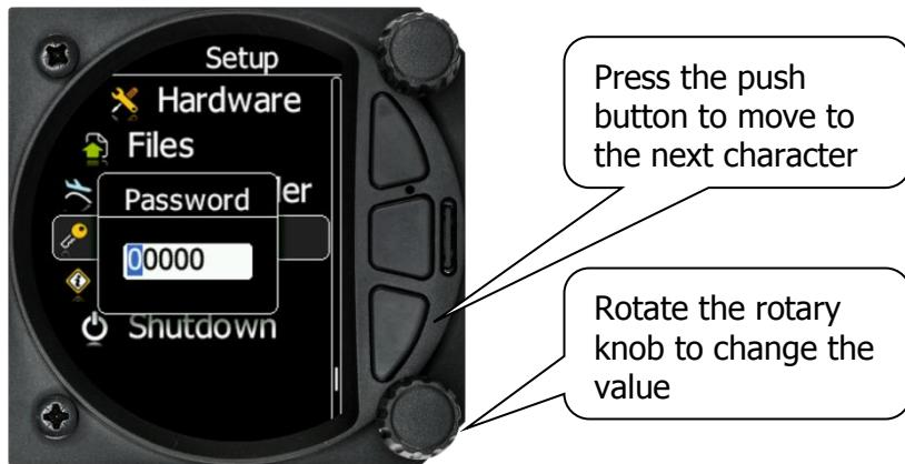
Once the required value is selected, press the lower push button to move to the next character selection. To move back to the previous character, press the upper push button. When you have finished editing, press the Enter key – the lower rotary button. A short press of the middle push button exits from the edited field ("control").
