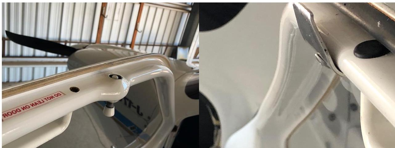
When talking to Jabiru pilots there will occasionally be a comment about the doors. Whilst they all have door locks – the models differ a bit when it comes to the top door latch. As we know, airflow tends to pull on the doors whilst in flight (moving the door away from the frame). The top latches are designed to prevent that happening.
